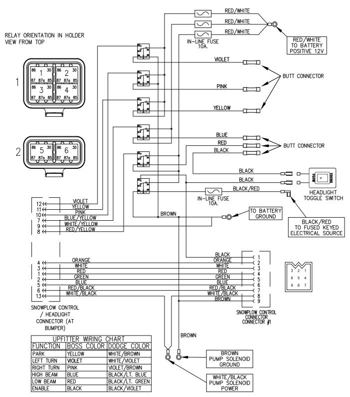
Truck Side Electrical Schematic (Rev. 0)
