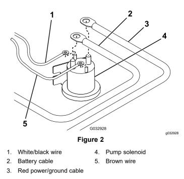
20. Connect the brown wire from the wire harness to the other small post on the pump solenoid.
