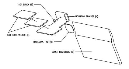
Figure 3 Mounting Bracket Vertical
