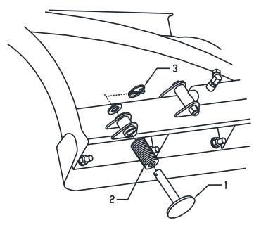
Figure 1. Plow Wing Shoe Assembly
