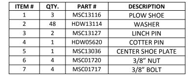
**Note:** This instruction manual is to be used for the installation of the ATV/UTV Plow Shoe Option Kit, **P/N:** MSC13032 for use on the 5'6" V-XT Plow.
