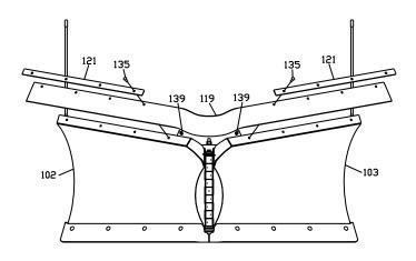
Figure 37. Snow Deflector Belting Assembly G10533
