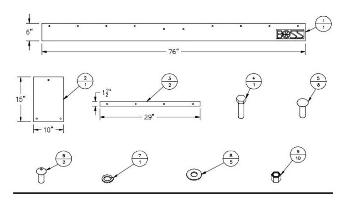
Figure 1. MSC13416 Snow Deflector and HDW13402 Fastener Kit Contents
