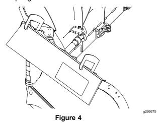
3. Using the holes in the plow blades as a guide, drill 9.5 mm (3/8 inch) holes through the belting.
