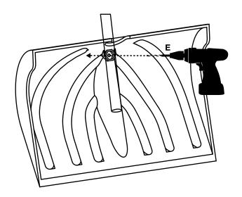
3. Insert Hex Bolt (1/4"x2") (D) in drilled hole and fasten with locknut (B).
