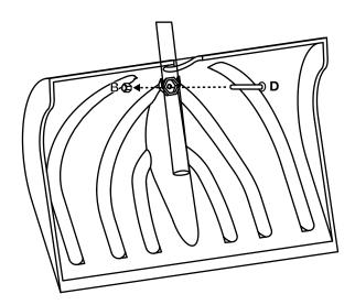
**4.** D-Grip should be parallel with blade - align by placing shovel on floor, before inserting self tapping screw (3/4") **(C)** into the handle.
