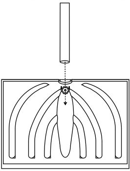
**2.** Drill a 1/4" hole in middle dimple with provided 1/4" Drill Bit **(E)**.
