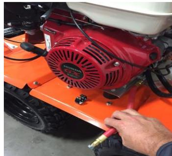
(pull drain plug to side of frame)
