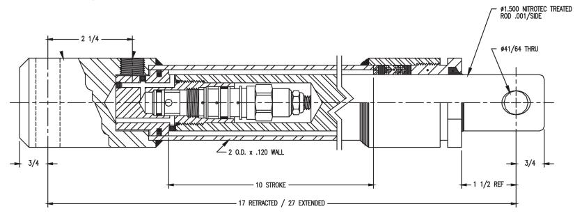
Service Parts: Seal Kit - HYD07035 Gland Nut - HYD07036 Piston - HYD07054 Valve - HYD07055
