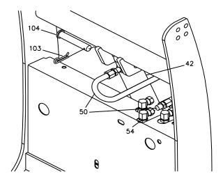
Figure 6. Assembly of Lift Cylinder Hydraulics.
