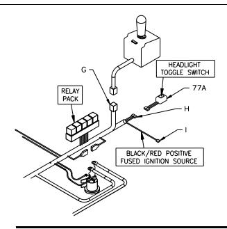
Figure 19. Internal Cab Wires
