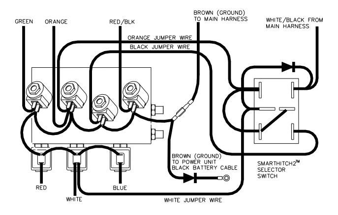
Figure 31. HYD07044 with SmartHitch2<sup>™</sup> Wiring Diagram
