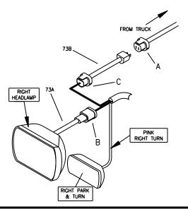
Figure 26. Single Headlight Adapter Connections
