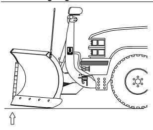
Figure 13. Front of Blade Not Level to Ground.
