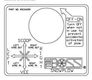
Figure 36. V-Blade Control Operation
