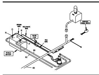
Figure 21. Battery Connections
