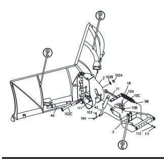
Figure 3. Push Frame Assembly Procedure.
