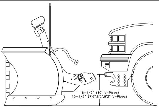
Figure 40. Recommended Push Beam Height
