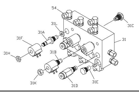
Figure 32. Hydraulic Valve Manifold Assembly.
