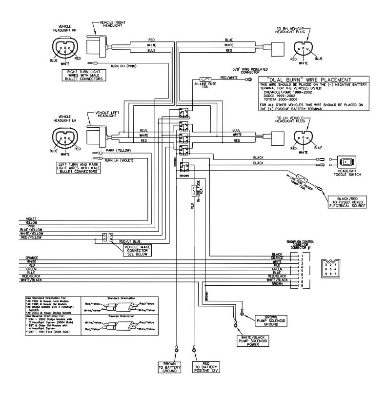
Figure 29. Electrical System Wiring Schematic (Truck Side)
