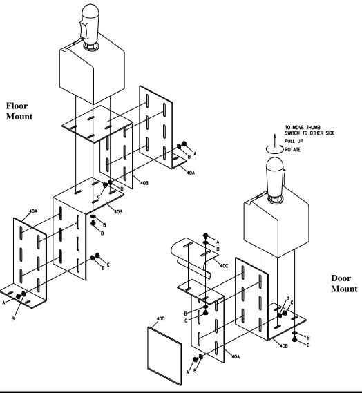
Figure 37. Joystick Control Universal Mounting Kit Components
