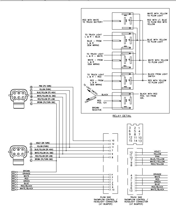
Figure 28. Electrical System Wiring Schematic (Plow Side)
