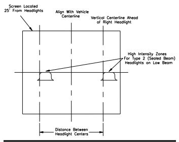
Figure 33. Headlight Aiming Procedure
