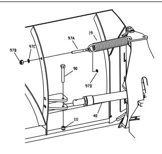
Figure 4. Angle Cylinder Installation.
