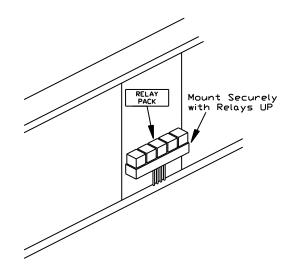
Figure 23. Relay Mounting.
