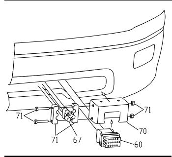
Figure 22. Vehicle Connections
