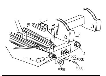
Figure 5. Coupler Assembly to Push Frame.
