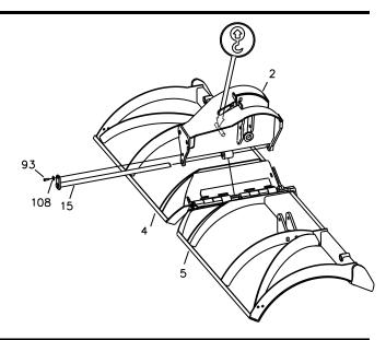
Figure 2. Blade Assembly Procedure.
