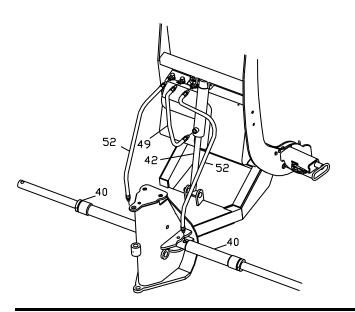
Figure 7. Assembly of Hydraulic Connections.
