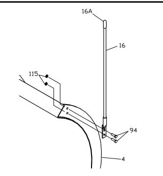
Figure 12. Assembly of Blade Guides.
