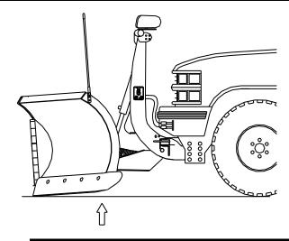
Figure 15. End of Wings Not Level to Ground.
