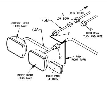
Figure 27. Dual Headlight Adapter Connections
