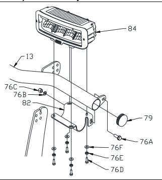
Figure 10. Headlight Mounting Assembly
