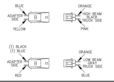
Figure 1. Headlight Adapter Orientation
