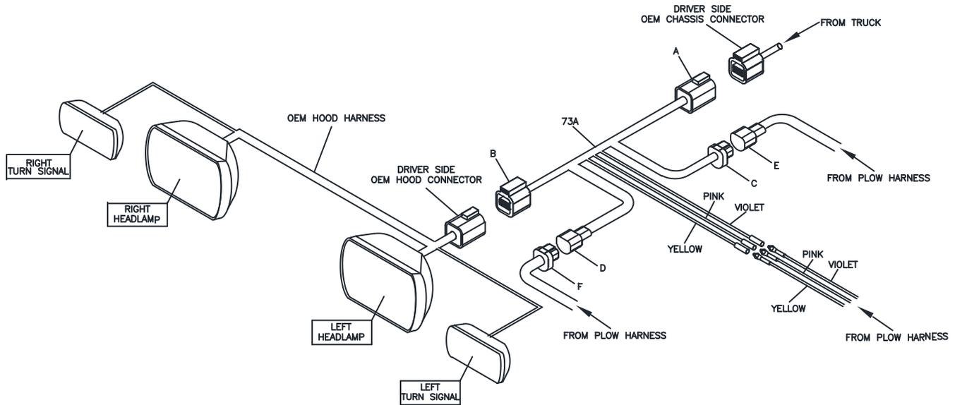
**Figure 1.** Ford F-650 & F-750 Headlight Adapter Installation
