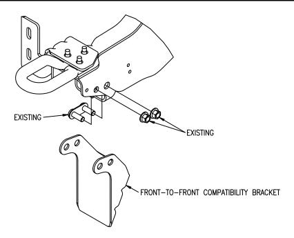
Figure 3. Front-to-Front Compatibility Bracket Removal
