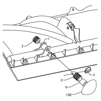
Figure 2. Plow Shoe Mounting Bracket Assembly G10315
