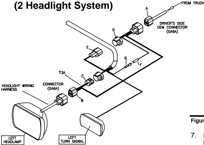
Figure 1. Driver's Side Single Connections G10372
