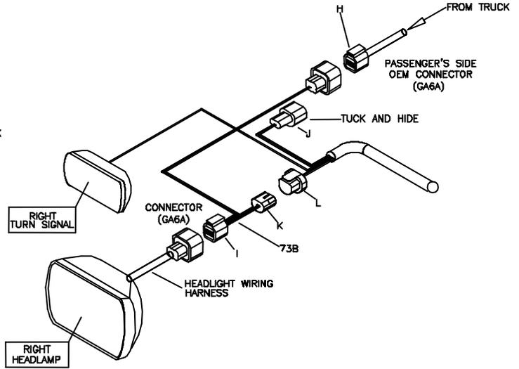
Figure 2. Passenger's Side Single Connections G10373
