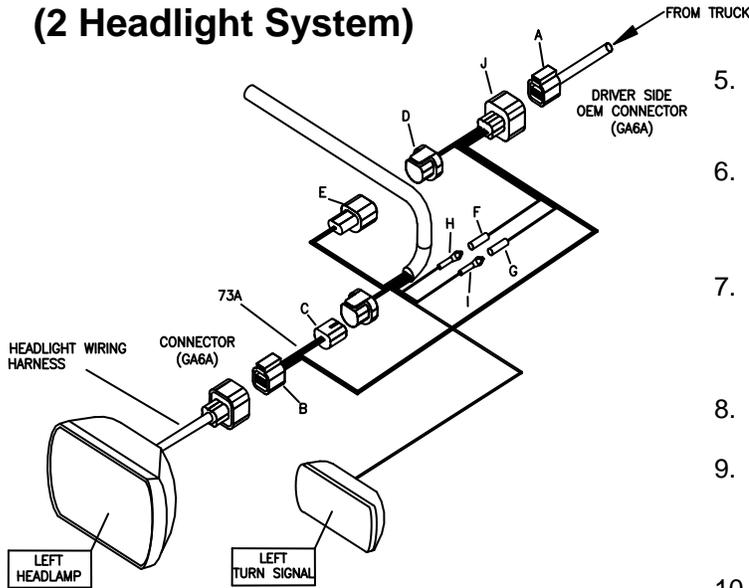
Figure 1. Driver Side Single Connections G10397
