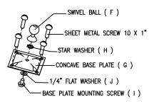
Figure 2 Concave Base Plate Assembly
