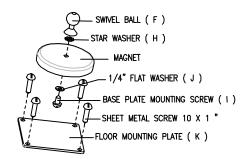
Figure 3 Magnetic Mount Assembly
