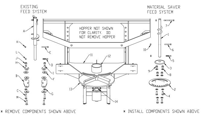
Figure 2: Existing Feed System Removal / Material Saver System Installation
