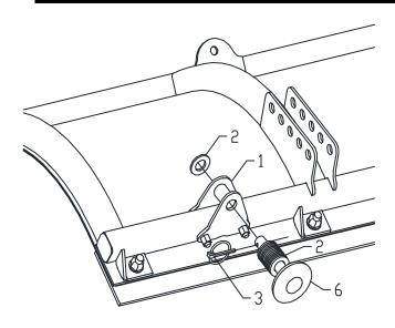
Figure 2. Plow Shoe Mounting Bracket Assembly G10923
