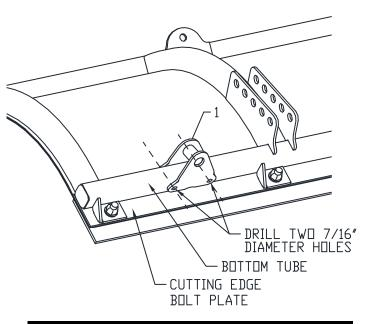
Figure 1. Drilled Holes Location
