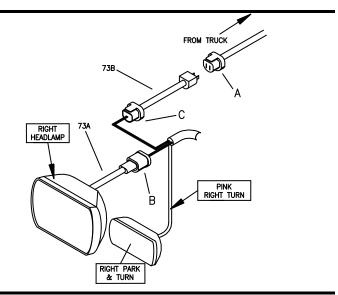
Figure 7: Single Headlight Adapter Connections
