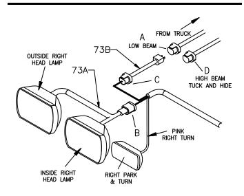
Figure 8: Dual Headlight Adapter Connections
