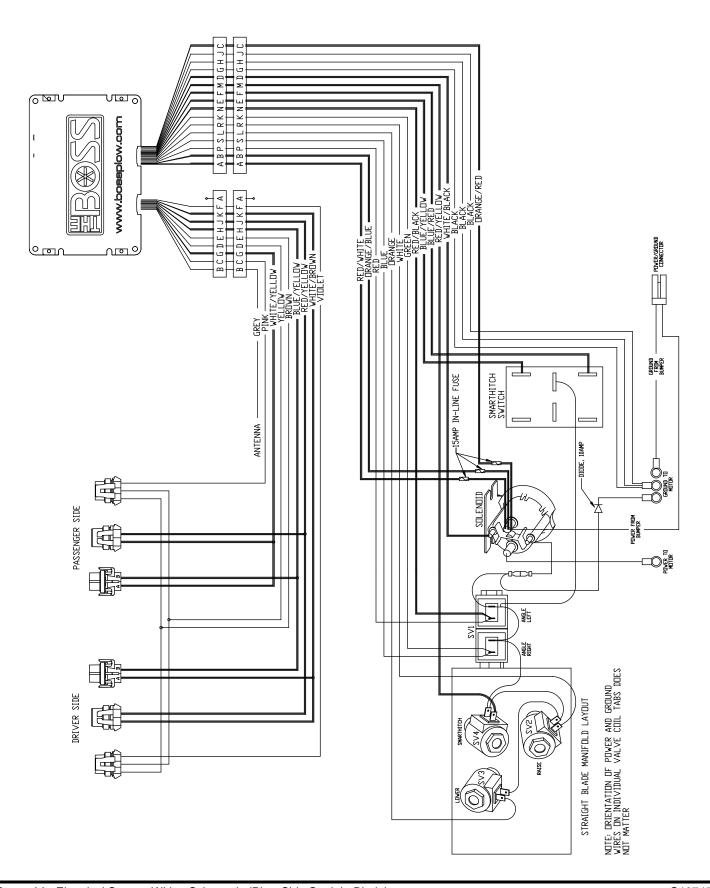
Figure 14: Electrical System Wiring Schematic (Plow Side Straight Blade)
