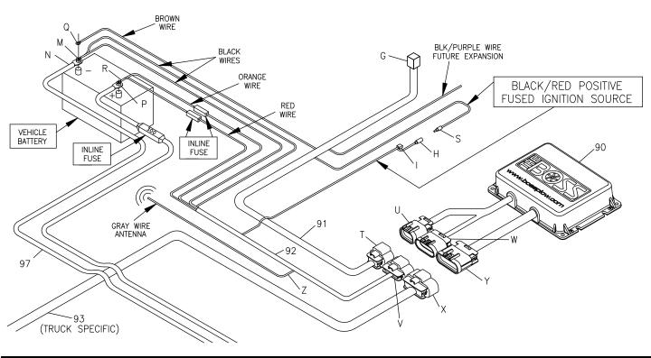
Figure 5: Internal Cab Wires
