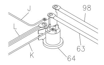
Figure 13: Solenoid Wiring
