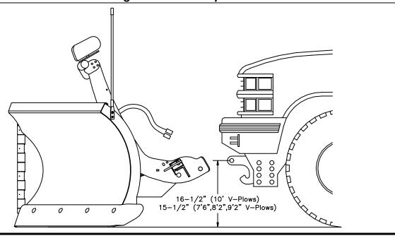
Figure 24. Recommended Push Beam Height
