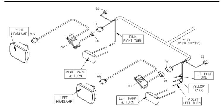
Figure 9: Headlight Resistor Wiring
