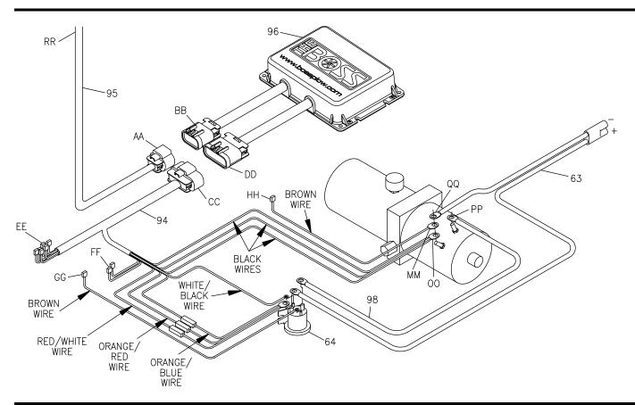
Figure 10: Plow Side Wiring
