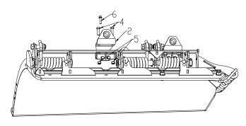
Figure 3. Plow Shoe Mounting Bracket Assembly G10828
