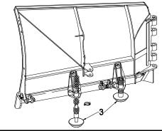
Figure 4. Plow Shoe Assembly
