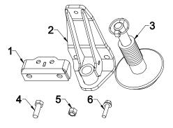
Figure 1. Bolt-On Shoe Bracket Kit Contents
