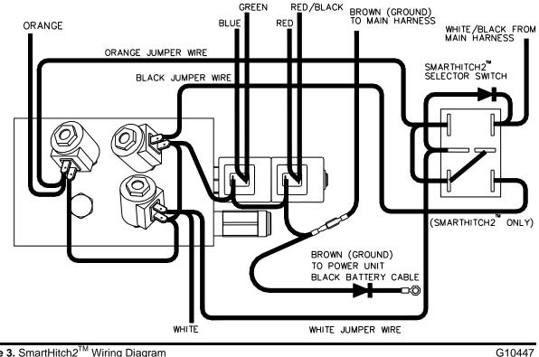
Figure 3. SmartHitch2<sup>™</sup> Wiring Diagram
