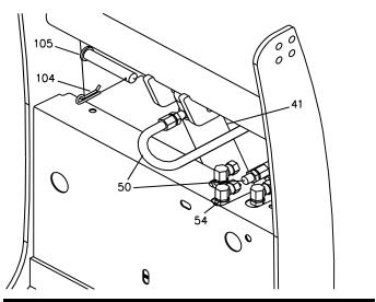
Figure 2. Installing SmartHitch2<sup>™</sup> Hose
