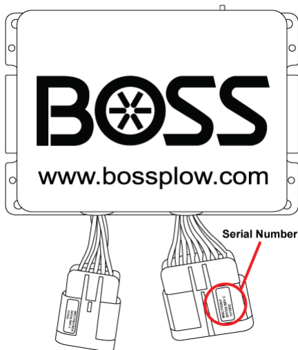
Figure 2. Serial Number and REV Level Location G13933
