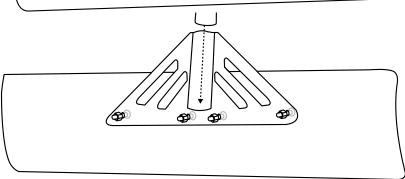
**4.** Drill a 1/4" hole in middle dimple on the backside of the TUFFBRACE with provided 1/4" Drill Bit **(E)**.
