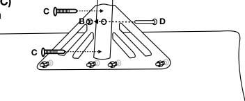
**6.** D-Grip should be parallel with blade - align by placing shovel on floor, TUFFBRACE side up, before inserting self tapping screw (3/4") **(C)** into the handle.
