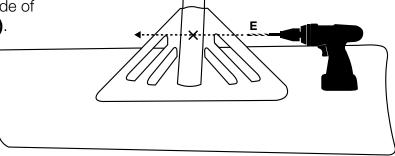
**5.** Secure handle to TUFFBRACE with 2 screws (3/4") **(C)** Insert Hex Bolt (1/4"x2") **(D)** in drilled hole and fasten with locknut **(B)**.
