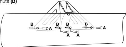
2. Insert remaining hex bolt (A) in the top blade hole and fasten to TUFFBRACE with locknut (B).
