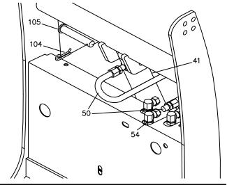
Figure 12. Installing SmartHitch2<sup>TM</sup> Hose
