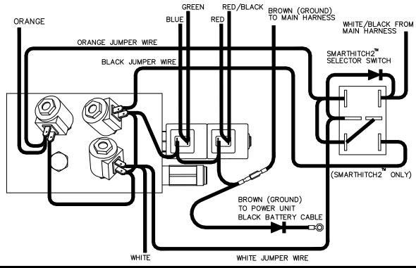
**Figure 13.** SmartHitch2<sup>™</sup> Wiring Diagram
