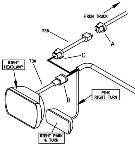
**Figure 24.** Single Headlight Adapter Connections G10149
