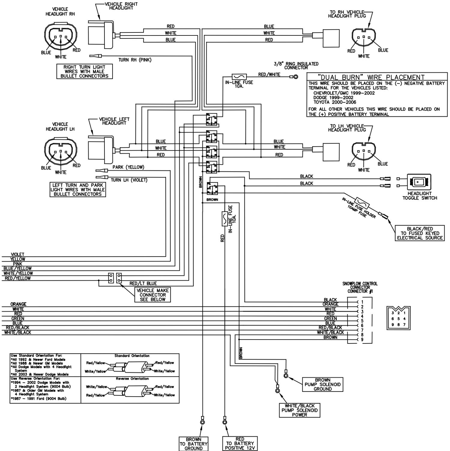
Figure 27. Electrical System Wiring Schematic (Truck Side)
