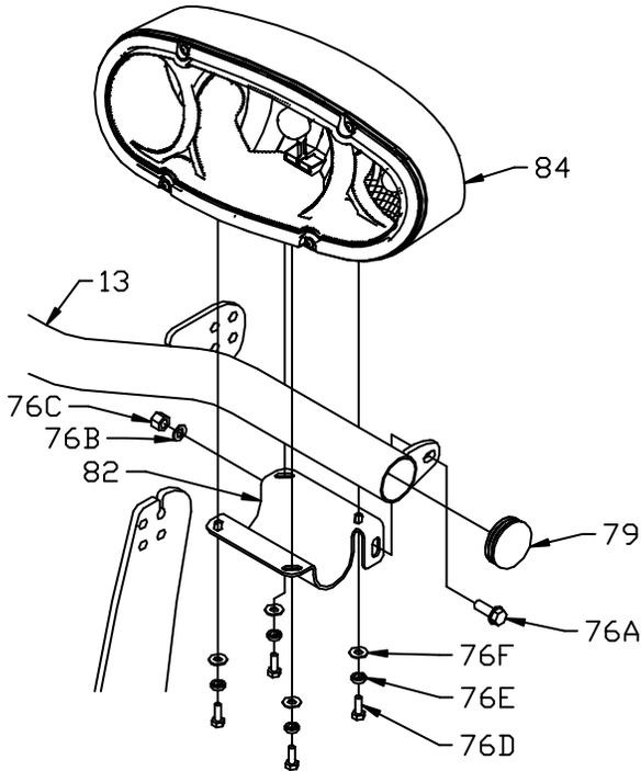
**Figure 8.** Headlight Mounting Assembly G10115
