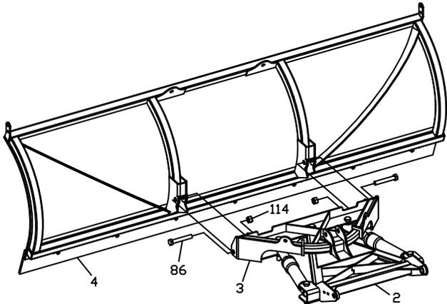
**Figure 2.** Push Frame Attachment G10298
