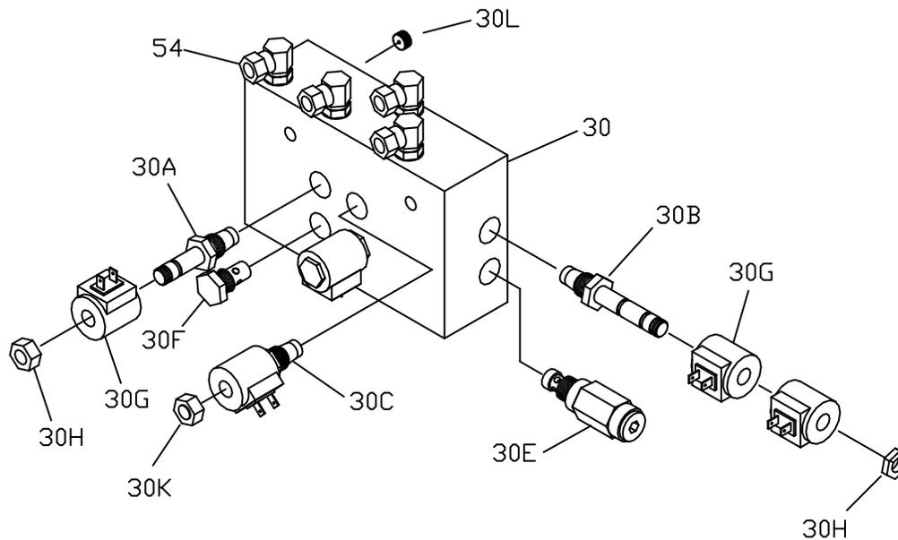
Figure 34. Straight Blade (Sport) Manifold with SmartHitch2™ Parts Diagram
