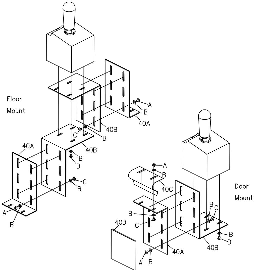
Figure 36. Joystick Control Universal Mounting Kit Component
