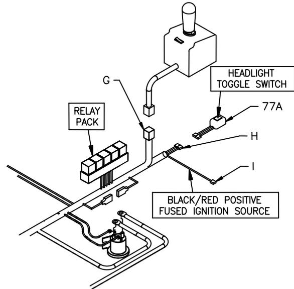
Figure 17. Internal Cab Wires
