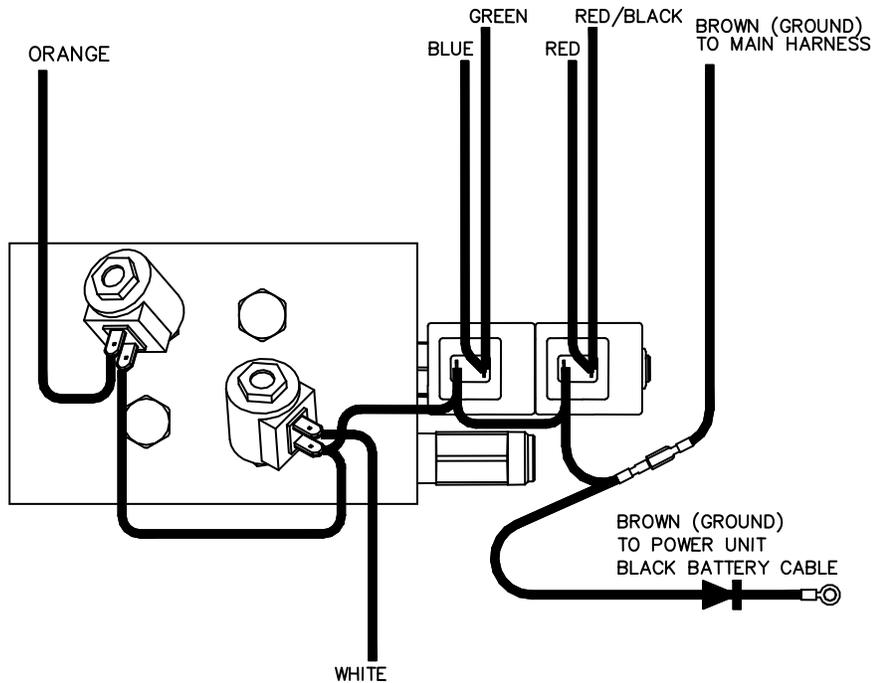
Figure 29. HYD07090 Sport Duty Manifold Wiring Diagram
