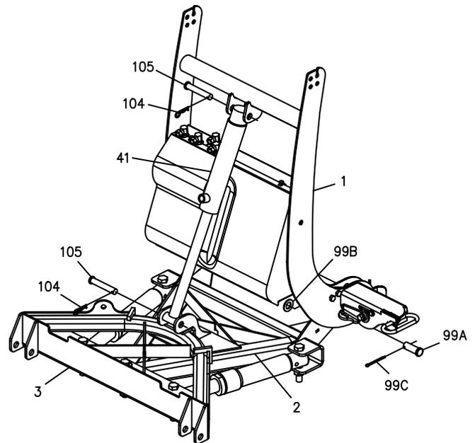
**Figure 4.** Lift Cylinder Installation G10301
