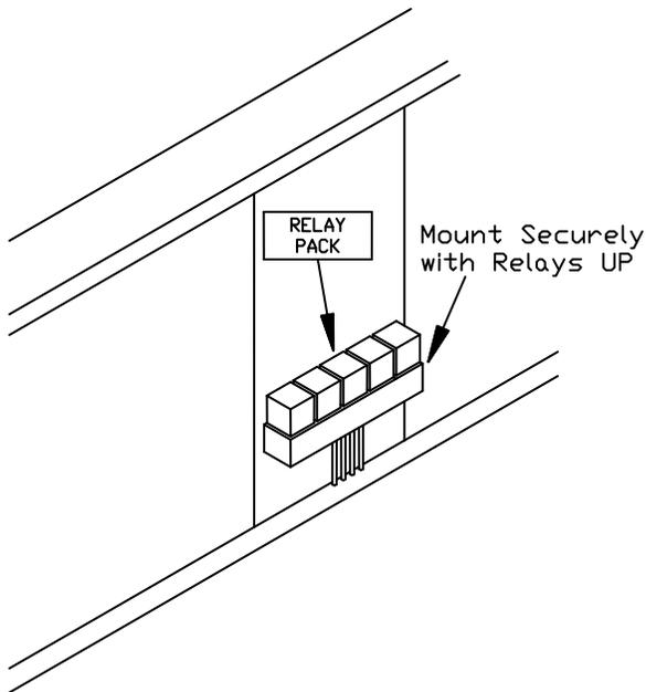
**Figure 21.** Relay Mounting.
