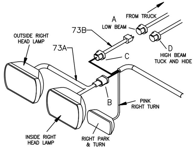
**Figure 25.** Dual Headlight Adapter Connections G10151
