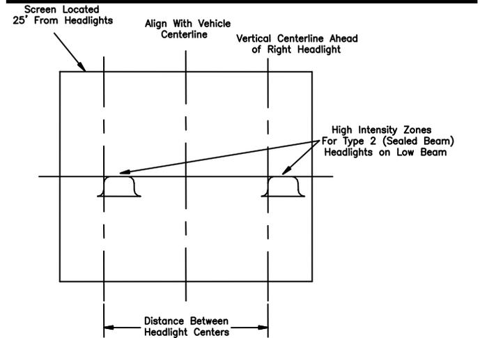
Figure 33. Headlight Aiming Procedure
