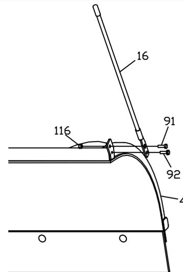
**Figure 10.** Assembly of Blade Guides G10304
