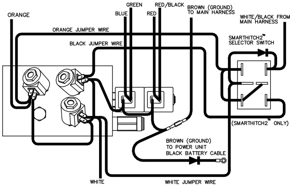
Figure 30. HYD07090 Sport Duty Manifold with SmartHitch2™ Wiring Diagram
