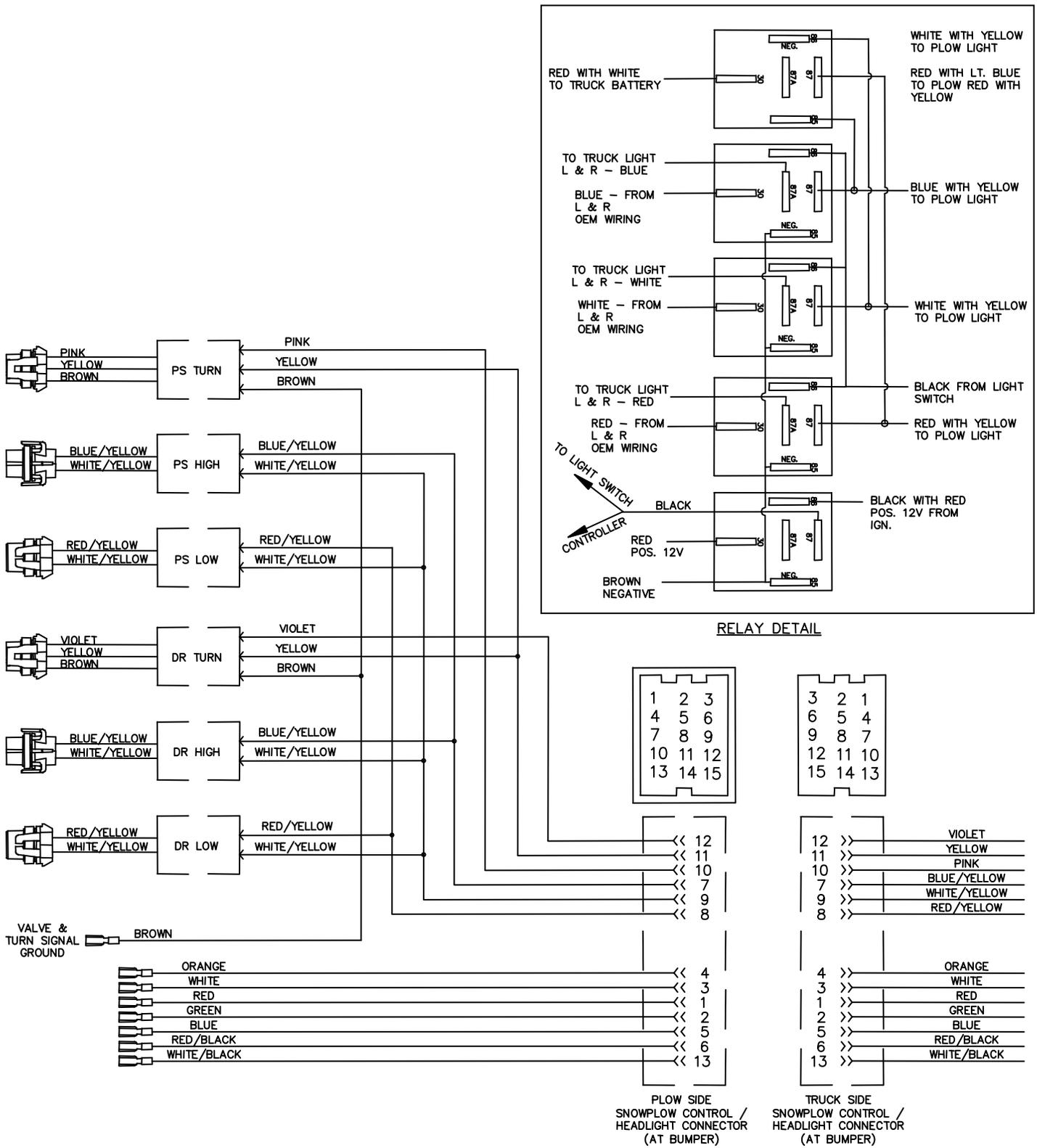
Figure 26. Electrical System Wiring Schematic (Plow Side)
