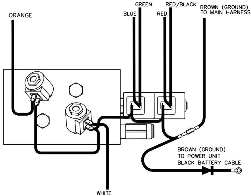
Figure 32. HYD07090 Standard Duty Manifold Wiring Diagram
