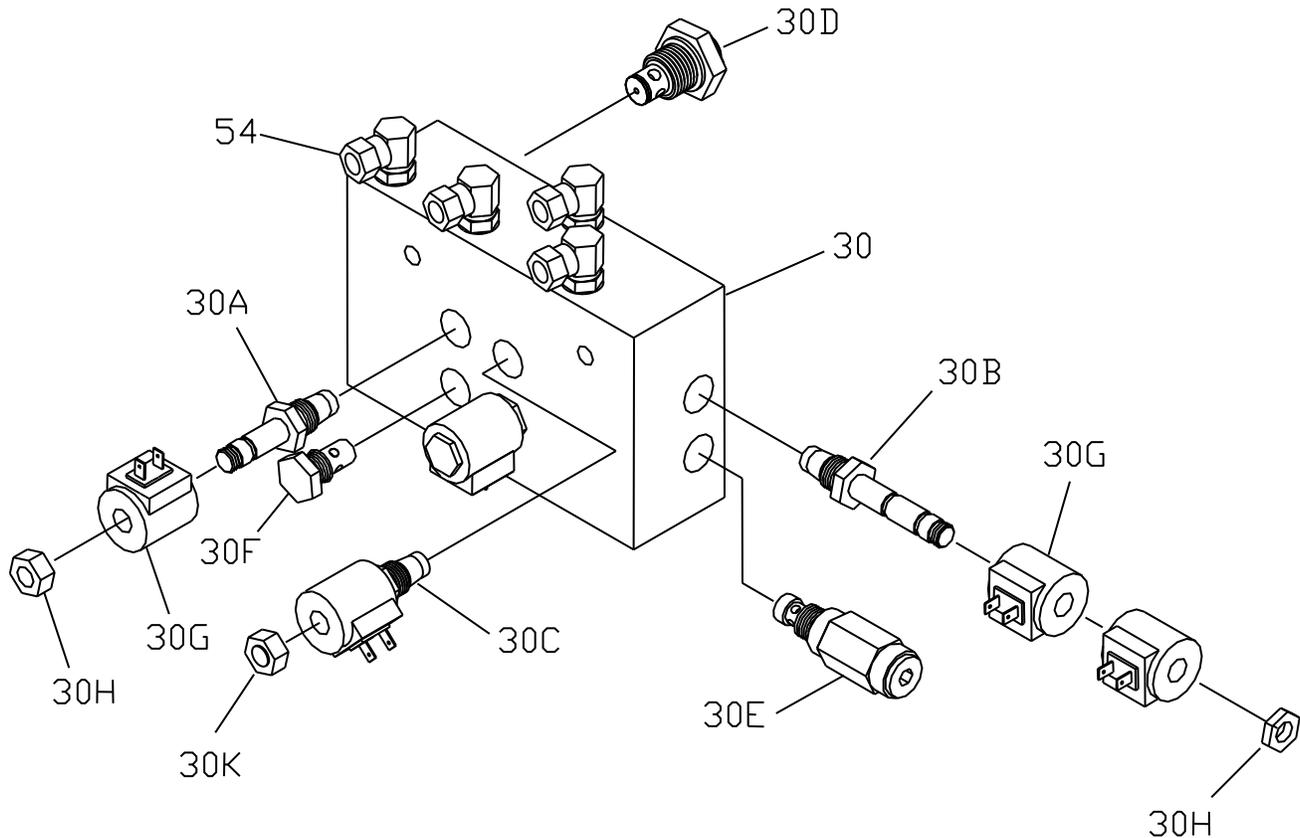
Figure 37. Straight Blade Manifold with SmartHitch2™ Parts Diagram
