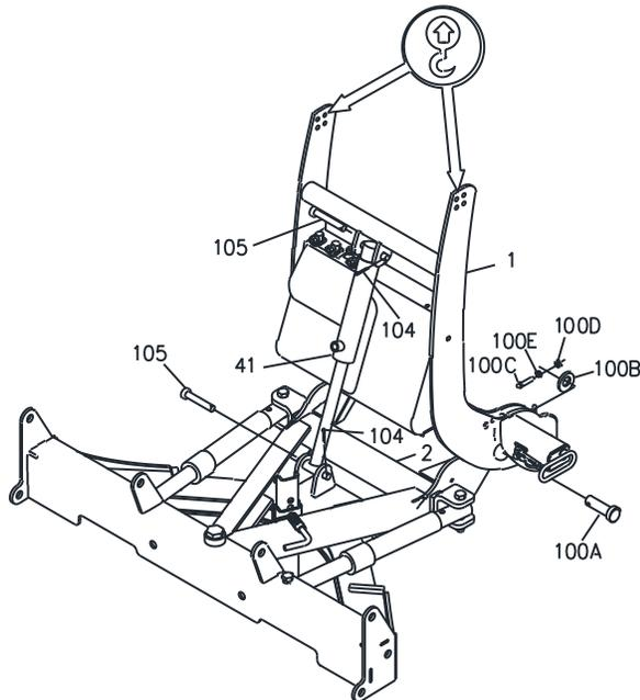
**Figure 6.** Lift Cylinder Installation G10110
