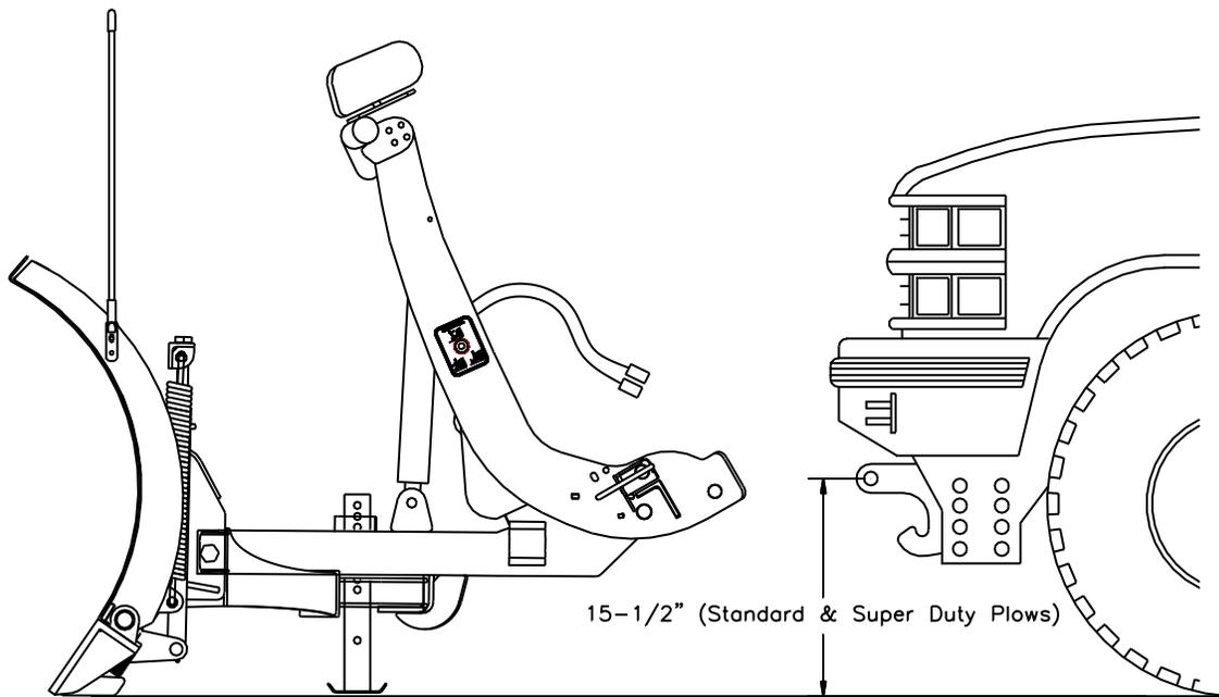
Figure 42. Recommended Pushbeam Height
