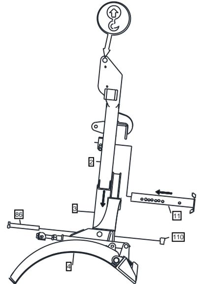
**Figure 4.** Install Pushframe and Kickstand. G10086
