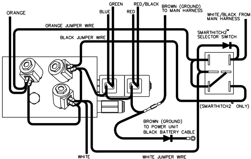
Figure 33. HYD07091 Super Duty Manifold Wiring Diagram
