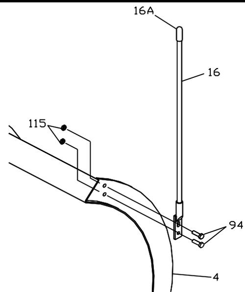
**Figure 13.** Assembly of Blade Guides. G10071
