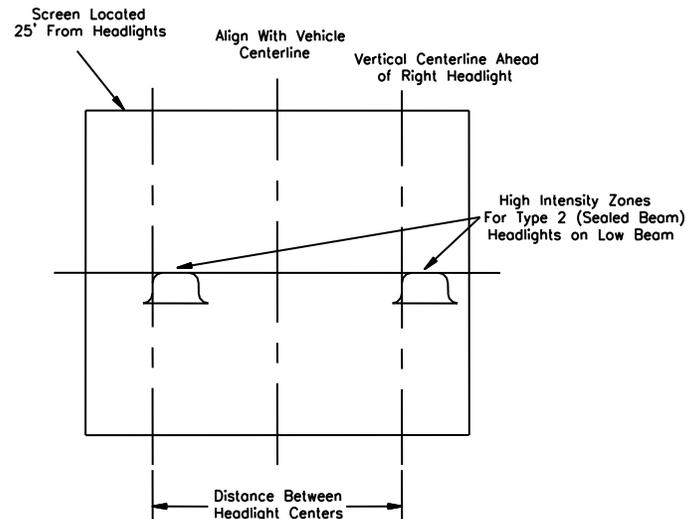
**Figure 30.** Headlight Aiming Procedure
