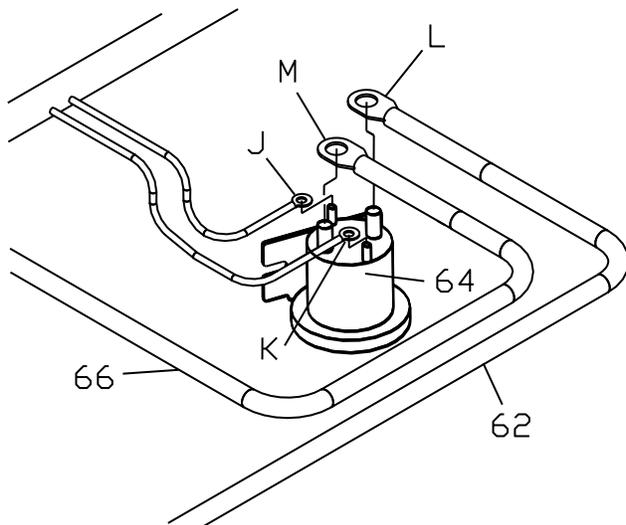
**Figure 21.** Solenoid Connections. G10145
