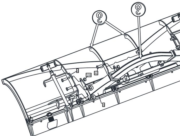
**Figure 3.** Install Pushframe Attachment Bar G10085
