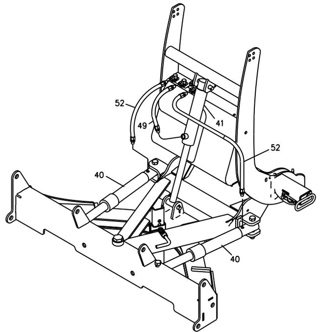
**Figure 7.** Hydraulic Connections G10111
