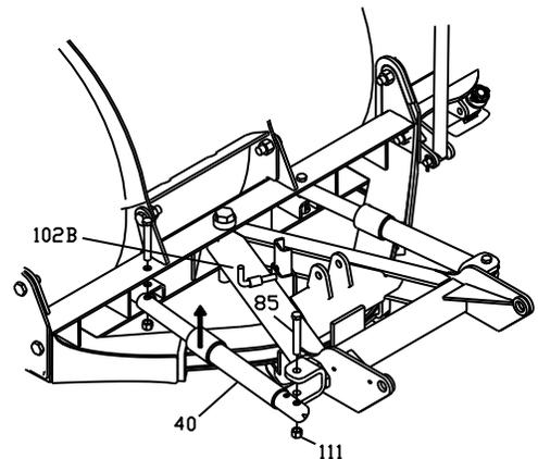
**Figure 5.** Install Angle Cylinders G10087
