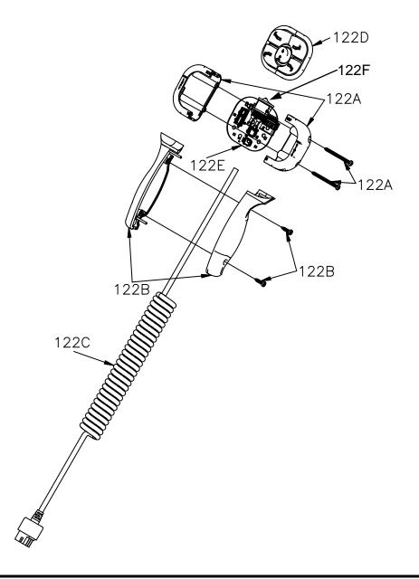
Figure 1. Power V-Blade SmartTouch2 Parts Breakdown
