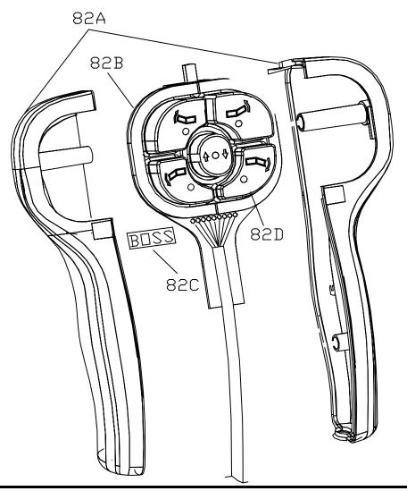
Figure 1. Power V-Blade Handheld Control Parts Breakdown
